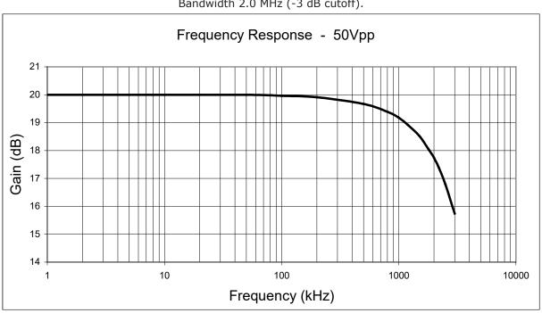
Figure 1: No Load and Full Load Gain (dB) vs. Frequency (Typical)
